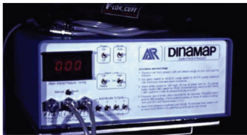
This early DINAMAP Instrument showed Mean Arterial Pressure (MAP) only.
